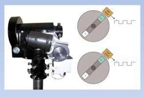
The very narrow HPBW ( about 3 Deg. ) requires strict control of orientation and the incremental encoders (Hall sensors) of SPID BIG-RAS/HR, together with the tower tilting mechanism, impose a re-alignment at the beginning of each session.
