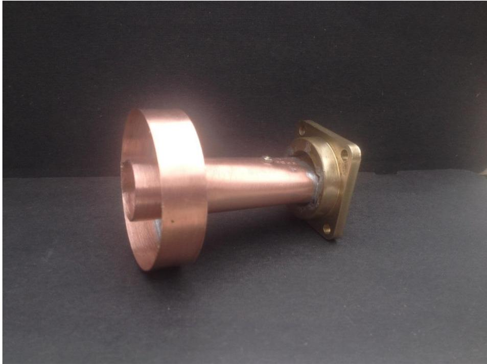
LP version of SM6FHZ's 0.692 wl feed constructed to (hopefully) have same illumination pattern as the CP feed and hence same dish efficiency.
